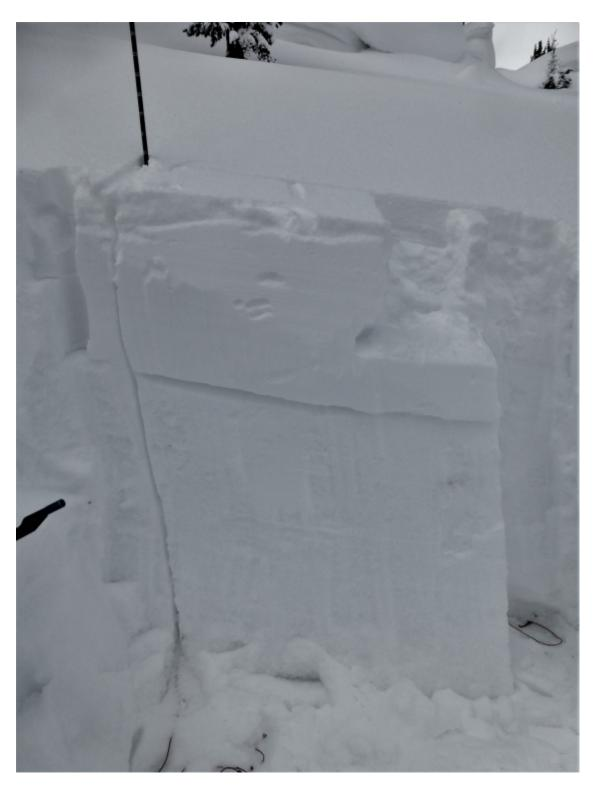
A layer of near surface facets was propagating in stabiliy tests on an east facing slope in Beehive Basin. It's worth digging and looking for this layer before committing to steeper slopes. Photo GNFAC
